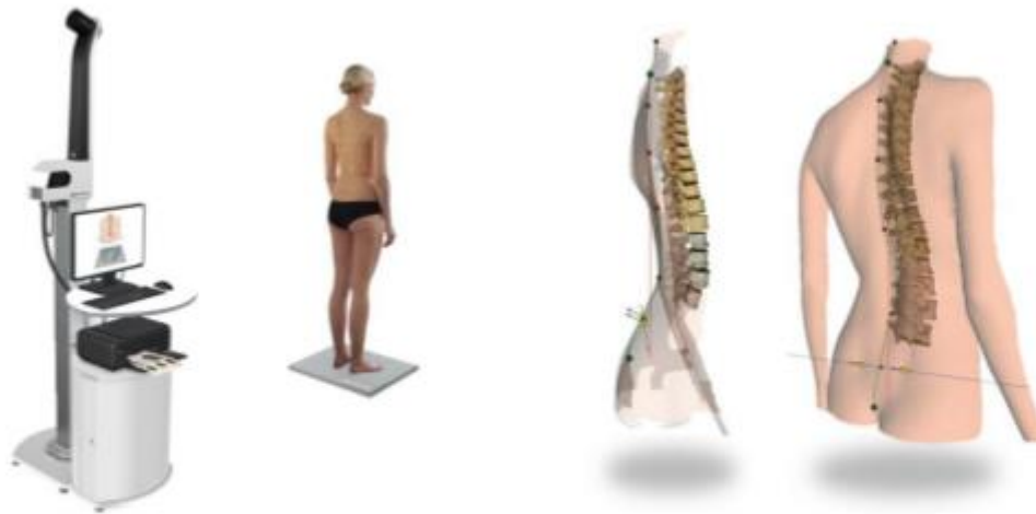
Fig. 1. DIERs Formetric system, and resulting 3D spinal reconstruction.
